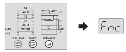
Press the [DRAWER] button several times until the lamp of the bypass tray is lit.
